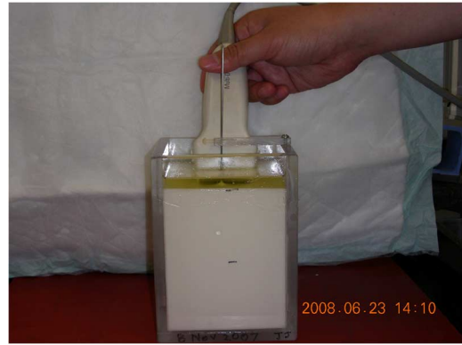
Fig. 2. Photograph illustrating data acquisition setup for the phantom experiment under freehand scanning. An imaging plane (typically 3 mm away from the needle electrode) is chosen to maximize the cross-sectional area of the spherical lesion without introducing reflection from the metal.
