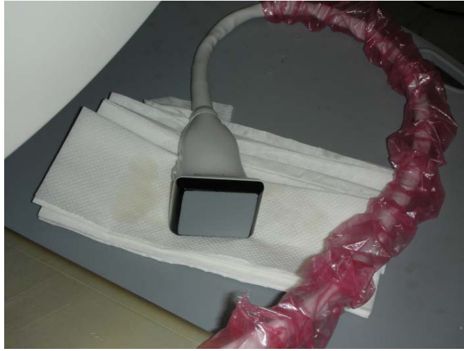
Figure 1. Prototype 2D CMUT array (courtesy of Siemens Medical Solutions, Inc., Mountain View, CA).
